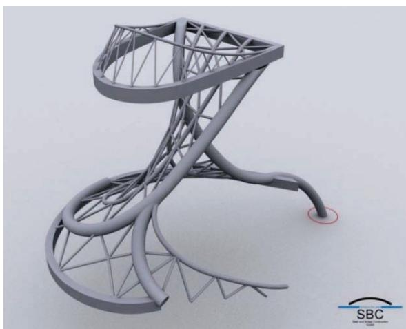
**Fig. 5** The steel structure of the Twist
