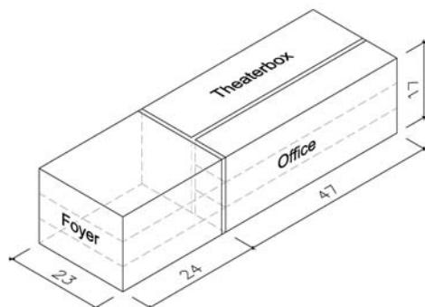
**Fig. 2** Main dimensions and functions
