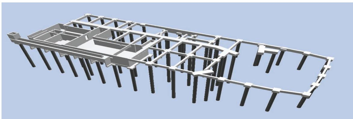
**Fig. 3** Piled foundation and parts below ground (Rendering: convex ZT GmbH)
