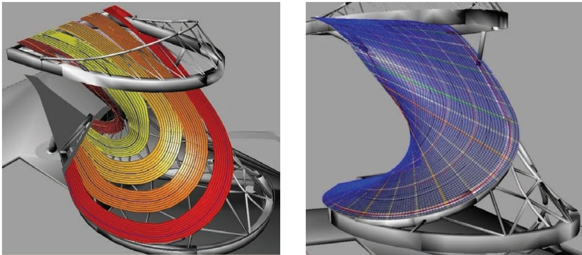
**Fig. 8** Longitudinal and cross reinforcement (Rendering: convex ZT GmbH)
