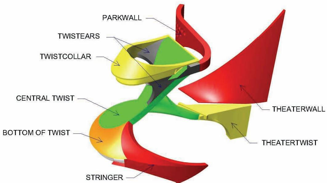
**Fig. 7** Coding of the Twist sections (Rendering: convex ZT GmbH)
